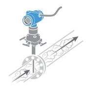
Annubar® Flowmeter accurately measures mass and energy flow with minimal restriction so that you can deliver more steam to your operation. ▶ p18
