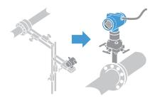
DP Flowmeters optimize performance by eliminating impulse lines to improve the accuracy and repeatability of your flow measurement, ensuring consistent product quality. ▶ p18
